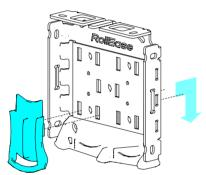
Push hooks thorough the bracket and pull down
