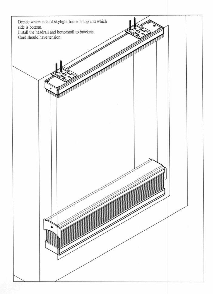
Install the headrail and bottomrail to the brackets. Operate the shade to make sure middle rail is leveled and cord has good tension. If cord is not tight, remove the bottomrail from the brackets. Loosen the cords from fix button and move the button upward. Tie the cord on fix button. Repeat the same process on the other fix button. Install the bottomrail on the brackets again to make sure the middle rail is leveled and operates smoothly.
