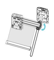
Push hooks thorough the bracket and pull down
