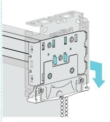
Push hooks thorough the Insert Plate and pull down
