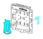
Push hooks thorough the bracket and pull down
