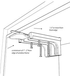
**Outside Mount:** Outside edge of the brackets should be positioned at a minimum of 2" from the outside of the headrail cassette, note the sticker on the headrail cassette. Use wall anchors for a secure hold. Mark the position of the bracket as illustrated.
